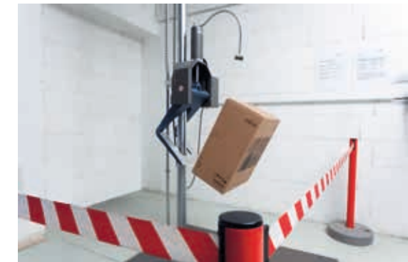
Drop test equipment
